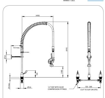
Spray gun position dimensions are approximate and represent a brand new unit, spring will sag with use over time
